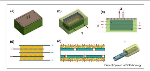
Design of an irrigating triple perfusion bioreactor.
